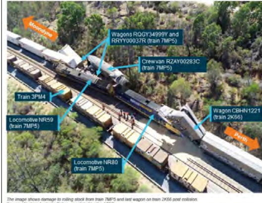
Figure 5: Accident site, lead locomotive of 7MP5 and last wagon of 2K66 post collision
